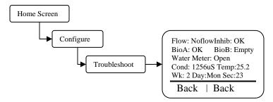
Flow – Water flow switch input (J4 pins 1-2).Flow=closed, Noflow = open.
