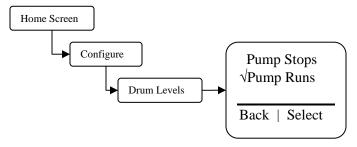
**Pump Stops** – Selecting this mode causes the inhibitor, biocide A, or biocide B outputs to de-energize when their drum level goes low.
