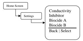
**Conductivity** – Set the conductivity setpoint, differential, probe calibration, alarms, and 4-20ma output parameters.
