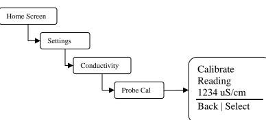
Step 1 – Move to the Probe Calibration screen.
