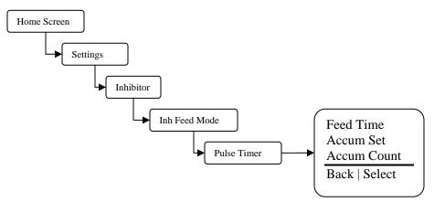
**Feed Time** – Set this value to the amount of time you want the inhibitor to feed when the water meter accumulator reaches its target.
