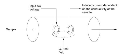
The main advantage of toroidal conductivity is that the toroidal coils are not in contact with the solution. They are encased in a polymeric material or are external to a flow through cell.
