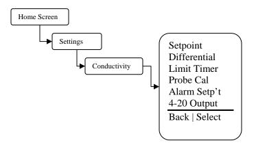
**Setpoint** – Set the conductivity setpoint. This is the conductivity point where a bleed function will begin. Once the conductivity has reached this value the bleed function will begin.
