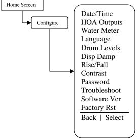
**Date/Time** – Set the current date, date format, time, and time format. **HOA Outputs** – Manually control the four output relays.
