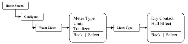
**Meter Type** – Select between a dry contact or Hall-effect water meter. Once the type is selected enter the resolution or volume per pulse.
