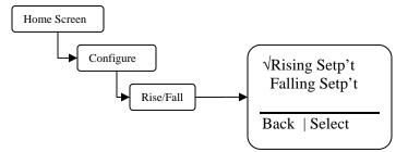
**Rising Setpoint** – Select this option if a cooling tower is being controlled. **Falling Setpoint** – Select this option if the conductivity tend to fall as a result of the
