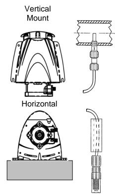
Figure 2: Injector Placement
