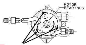
WARNING: Note severe pinch points between rollers and pump housing
