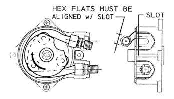
Figure 9c: Finishing the New Tube Installation
