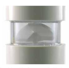
The triple turbine (patent pending) in the new inline mixer model induces the turbulence needed for increased mixing performance with a decreased differential pressure. This triple turbine changes the directional flow of the fluids, allowing mixture prior to exiting the mixing chamber.
