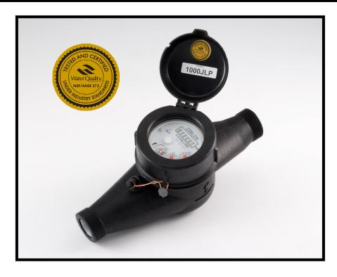
The JLP series is WQA/NSF 372 listed. This no lead meter is designed for aggressive water such as reverse osmosis and de-ionized. When long life, low maintenance and high accuracy are needed in a plastic totalizing or pulse out water meter, Carlon's JLP plastic meters are what you want. The JLP series comes in three sizes, 1/2", 3/4" and 1" and operates at flow rates from ½ GPM to 50 GPM and pressure up to 100 psi.
